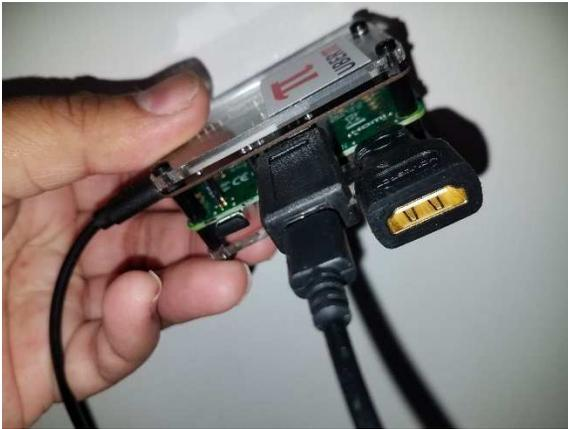
1. Plug in the HDMI cable into the unit via the mini HDMI to HDMI adapter and into an available spot on your television. If you have a cable that goes from mini HDMI to HDMI you are welcome to remove your adapter.
