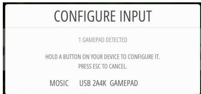
4. To configure your game controller, once in RetroPie hit Enter on your keyboard. Go down to Configure Input with the directional buttons and hit the A button. Configure your game controller per the instructions on the screen. Push and hold any button to begin, and then push the correct buttons as they are listed. To skip buttons, press two buttons and hold at the same time. When prompted about a hotkey, skip it. Then choose the option to make the select key your hotkey.
