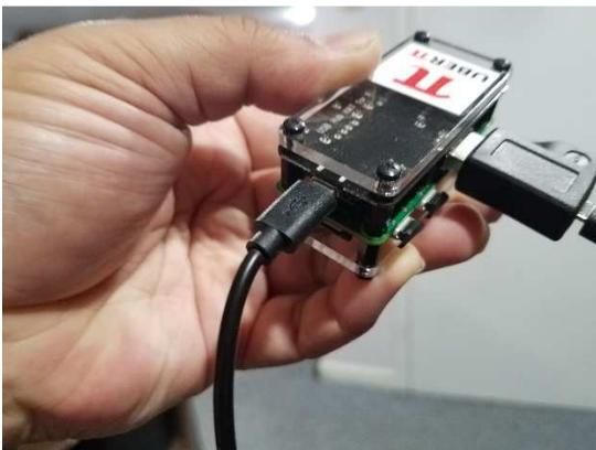
3. Put in your micro SD card THEN plug in the power cable only after numbers one and two are done. This will power up the unit and boot directly into RetroPie. The Raspberry Pi Zero will not boot if there is no micro SD card in it.
